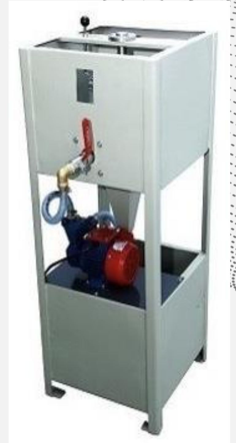
Jominy Hardenability Test Apparatus
