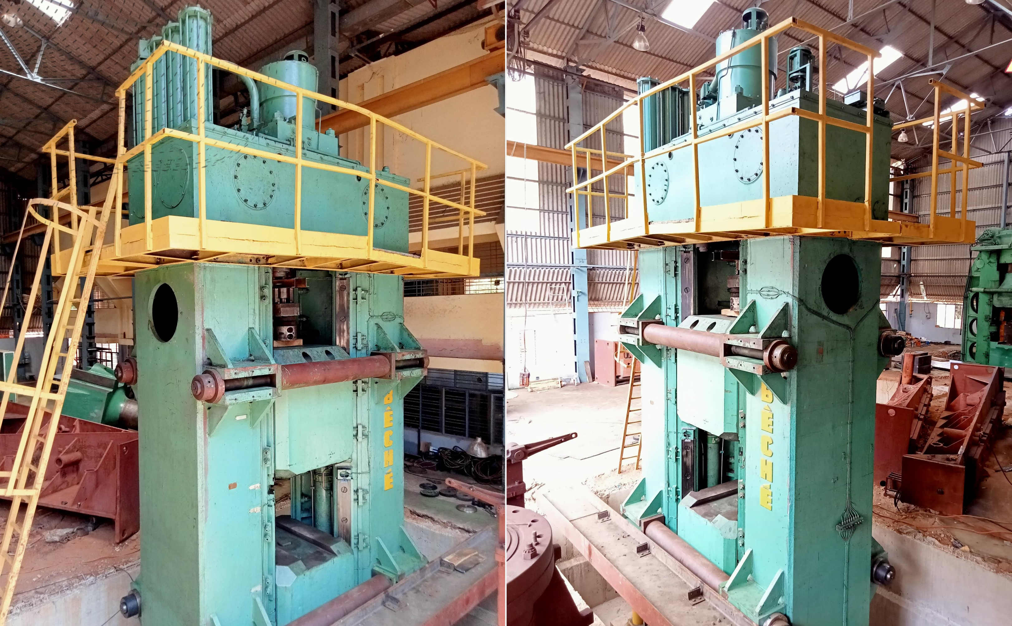
13 T Hydraulic Counter Blow Hammer – Beche HG 13
