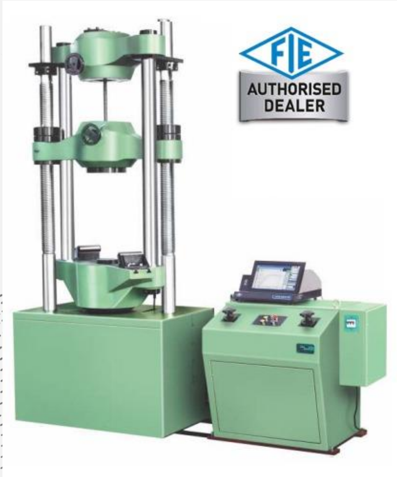
20 T Universal Testing Machine - Electronic
