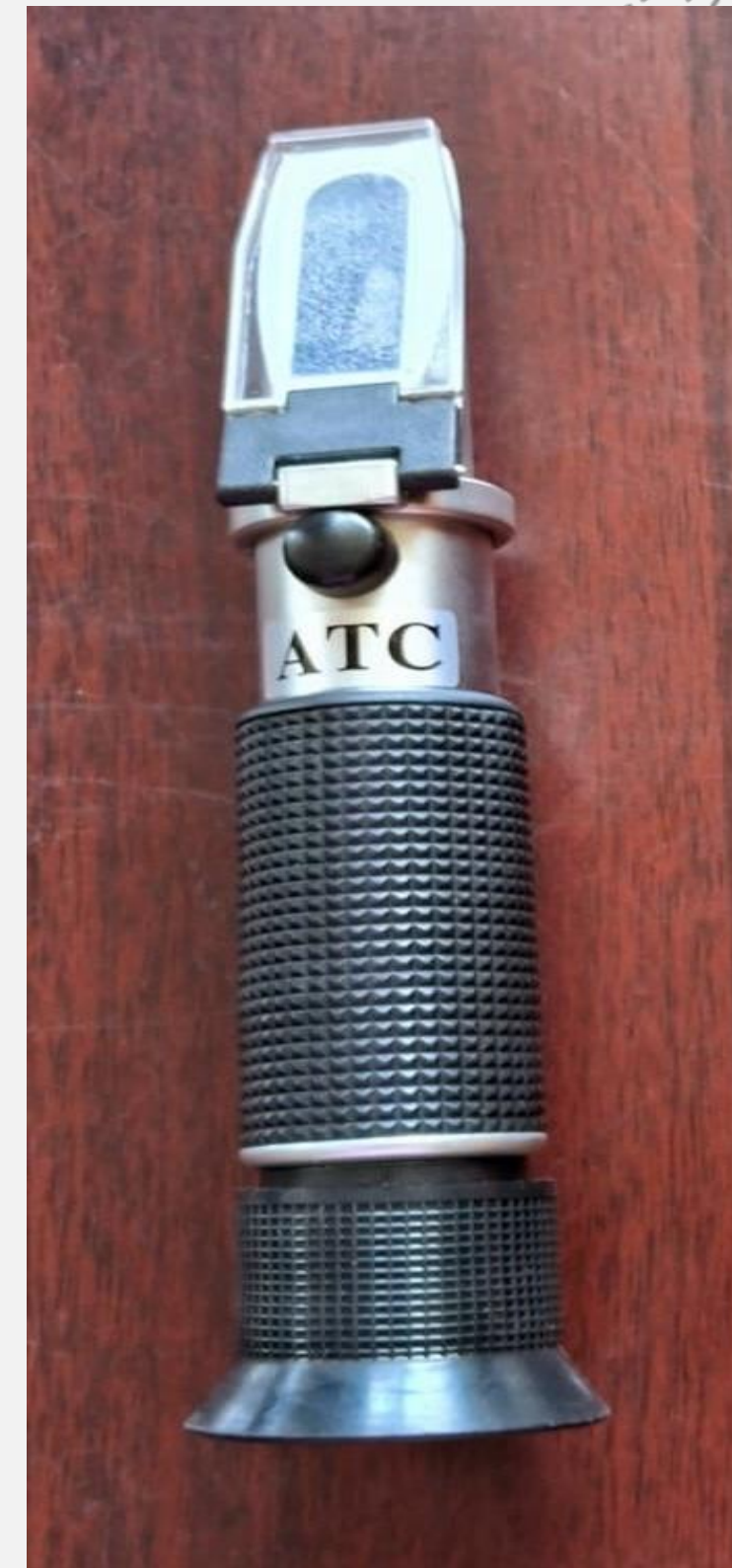
Refractometer for Checking Strength of Polymer bath
