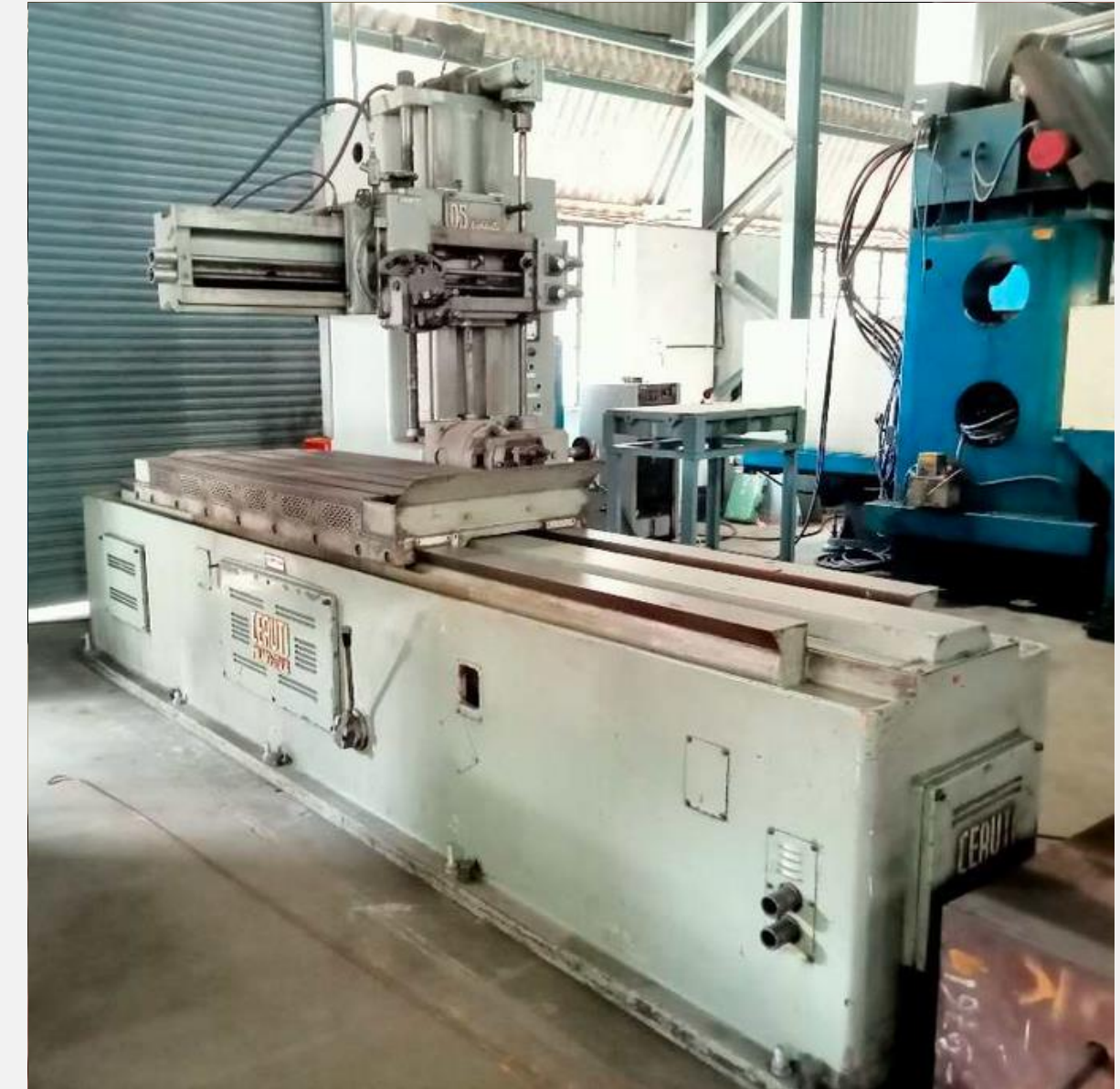
Planing Machine 1500 x 500 mm
