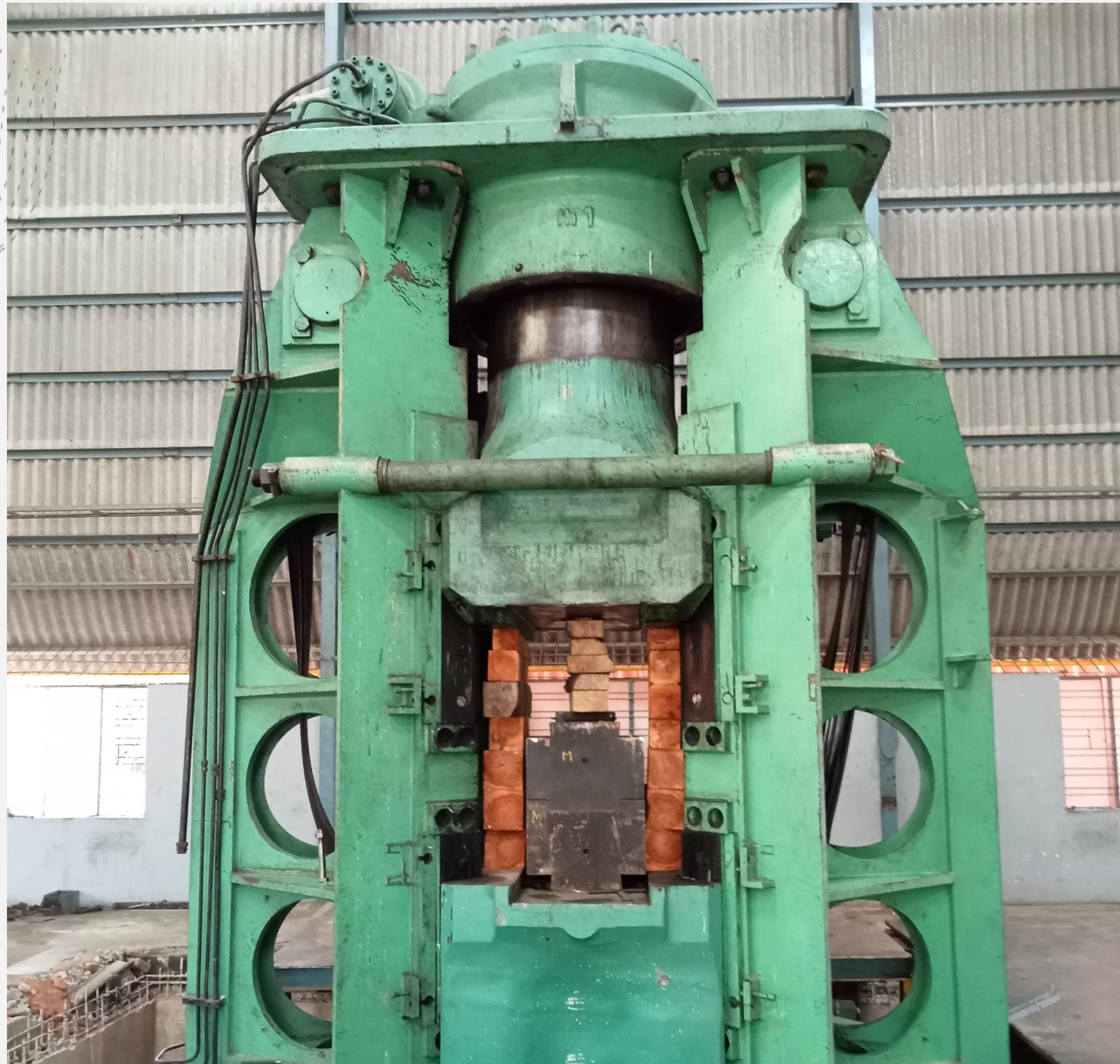
32 T Counter Blow Hammer - Beche DG 32
