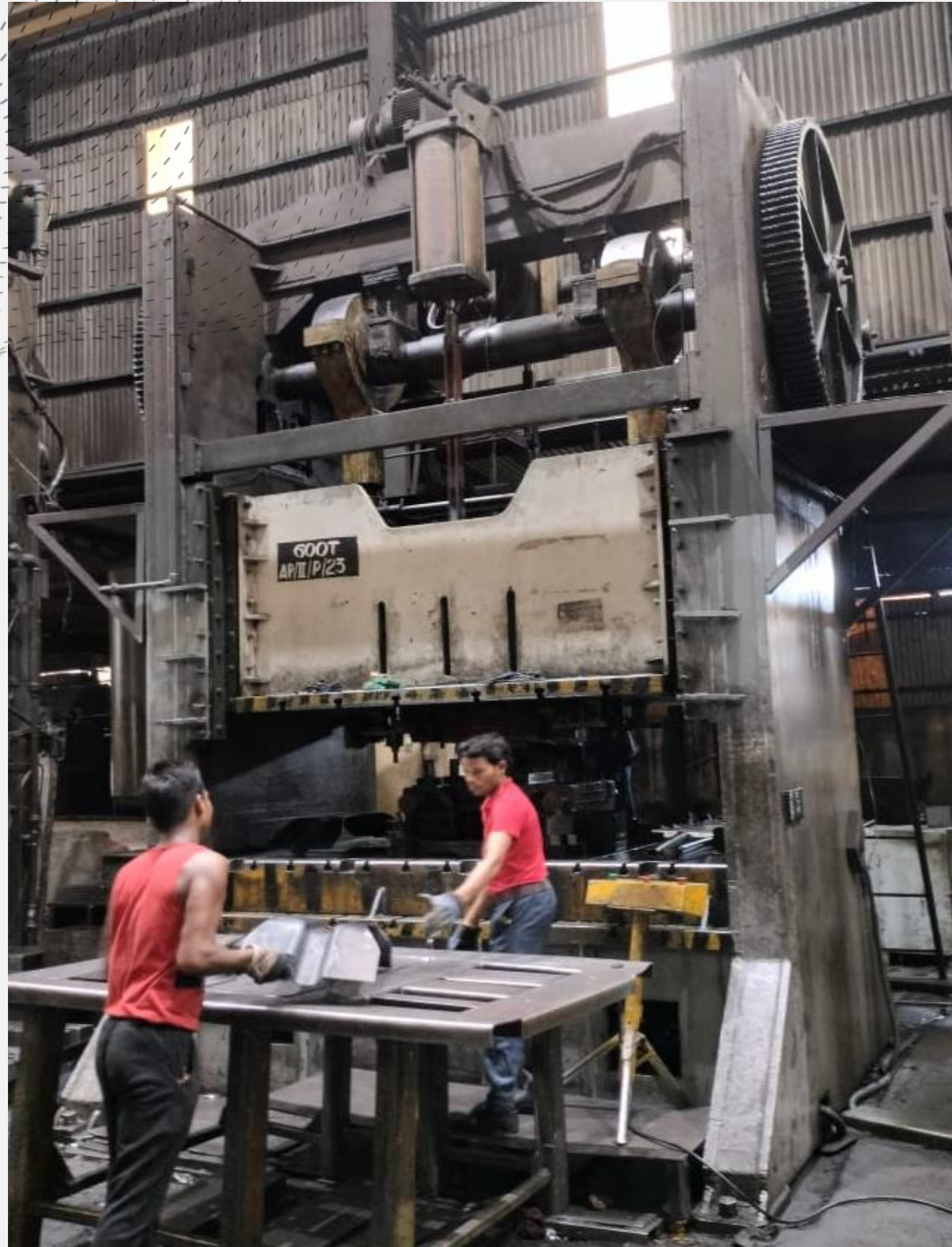
600 T Weldor Trimming Press
