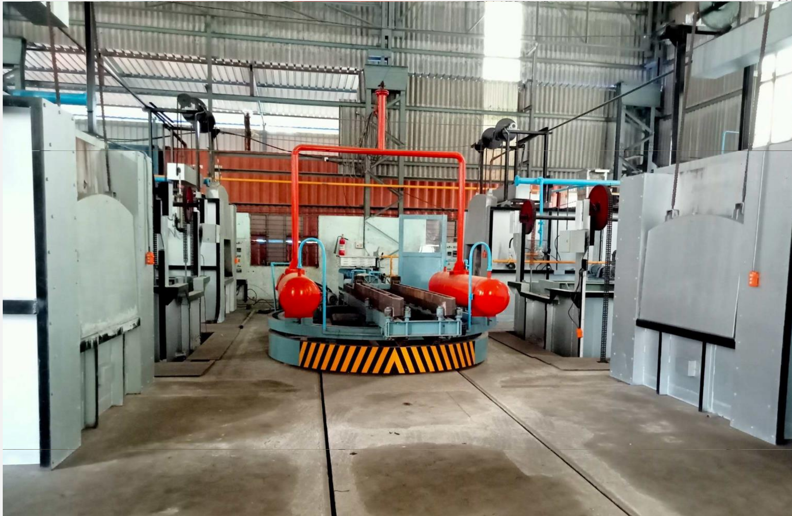
Semi Automatic Charging Machine for Unloading and Transfer of Hot Forgings from furnace to Quenching tanks ( Polymer and Water within 45 Sec)
