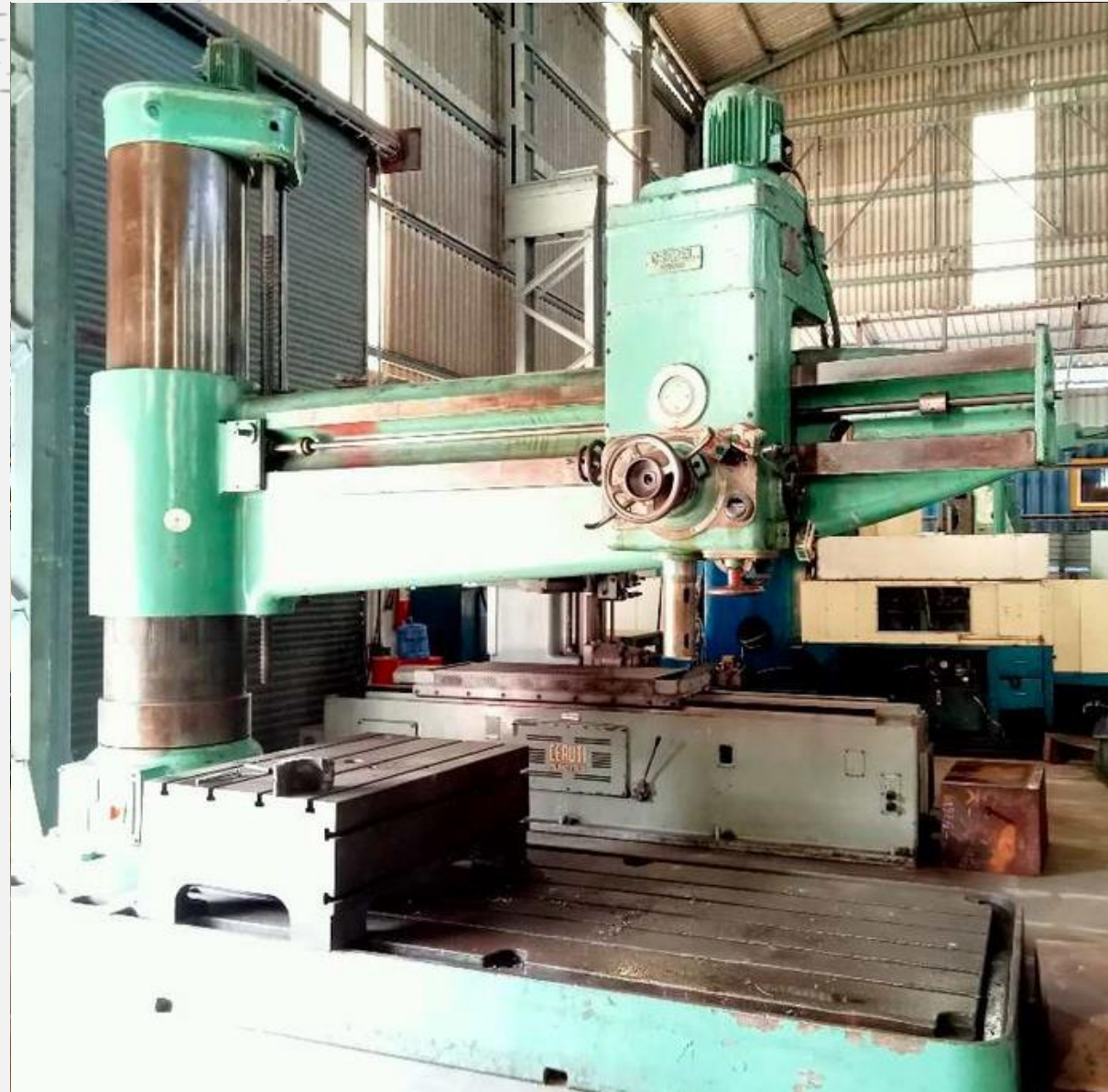
Pillar Drilling Machine Drilling Capacity 90 Dia Arm Length 3 Mtrs
